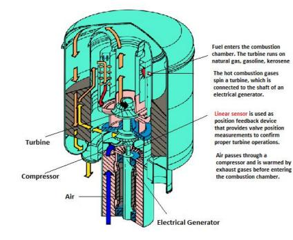
Linear Sensors are used for measuring the position of the operating shafts of turbine control valves and also as the position feedback device that provides valve position measurements to confirm proper turbine operations.
